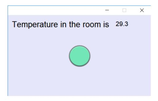
The last missing step is the address on the button. Double click the button and on the **Set Bit Object's Properties** change the **Write address** device to the UniPi controller, **Address** to **0x** which is a designation of "coil" and the coil number leave at **1**.
