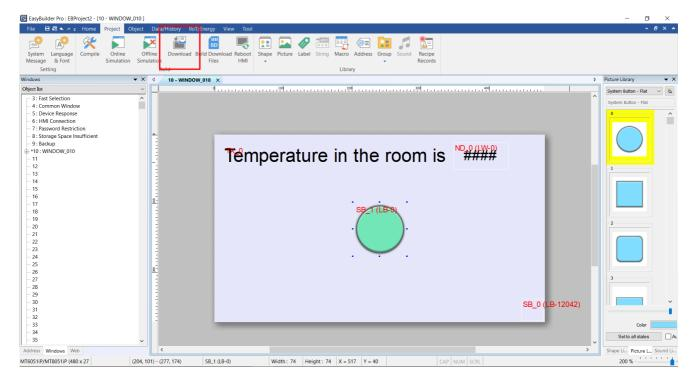
The only operation you have to do in the **Download** dialog is filling the IP address. Then hit **Download**. The HMI device will reboot and start your project. The result should look the same as in the simulation. The temperature will be 0 and pressing the button does nothing.
