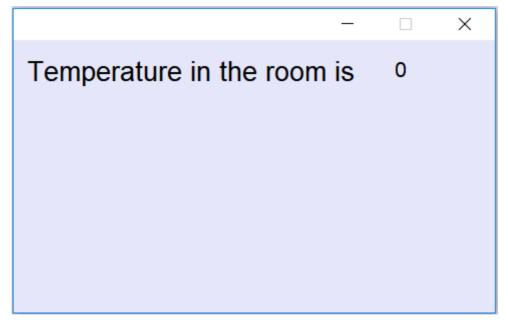
So far we have created simple window, which displays a numeric value of some register. To make this tutorial little bit more versatile, let's learn, how to create a button, which - in the end - will operate relay output on our UniPi. To do this, we have to place new object onto the window canvas, called **Set bit**. On **Object** panel, click on the **Set bit**.
