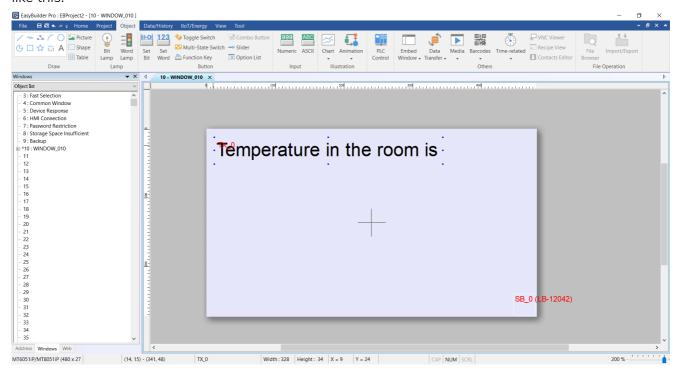
The text object is static, which means the content cannot be dynamically changed e.g. from some variable or register. For displaying content of local HMI variable or Modbus register, we have to add numeric display box. Click on the **Object** panel on the **Ribbon** and then select **Numeric** in **Input** section.
