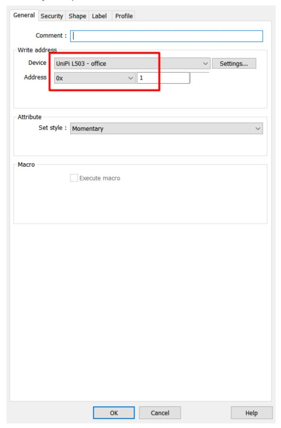
Run the **Online simulation** and try pressing the button. If you set it to relay output in Mervis, you should hear the clicking sound of the relay. If you set it to digital output, the LED on the controller should be turning on and off.
