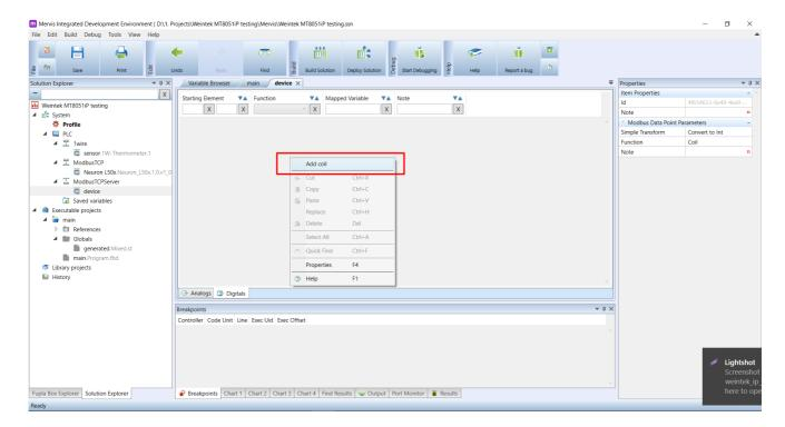
Double click on the **n/a** under the **Mapped Variable** and type **RO.2\_01**. If you don't have relay output 2.1 on your unit, you can type DO.1\_01. Select the found variable in the list.
